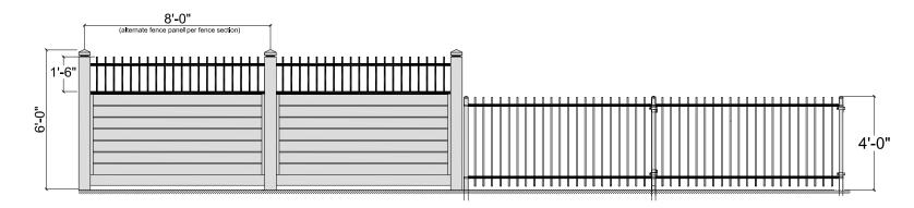
Solid Fence with Open Style Top - Street or Path Side Yard Elevation -Typ.
